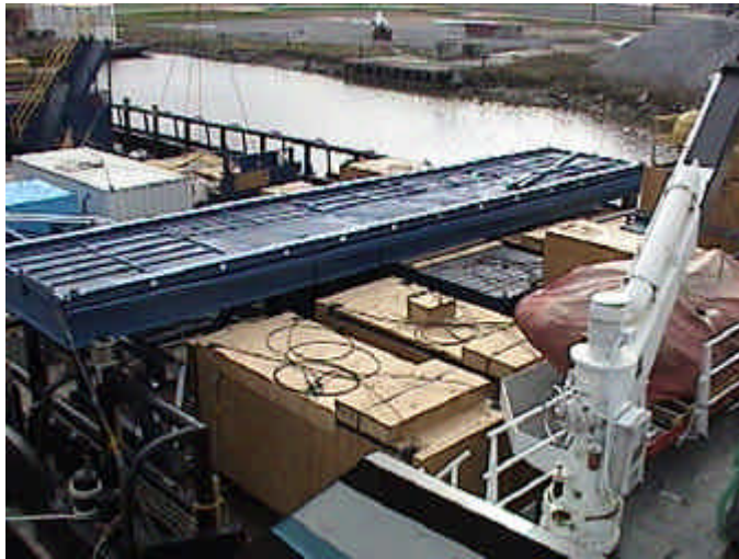
Complete Rig, piperack and quarters loaded onto typical Gulf of Mexico workboat With 130 ft x 45 ft deck space
